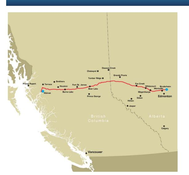
Enbridge has applied for federal approval to build the 728 mile Northern Gateway pipelines, which if approved would transport 525,000 barrels of oilsands products per day via a port in Kitimat, B.C.
