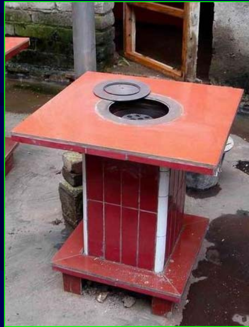
Movable coal stove made of brick and iron fittings
