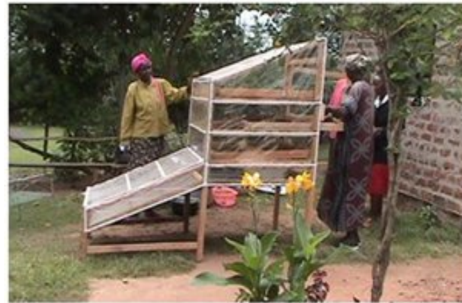
Improved indirect solar dryer (Kenya)
