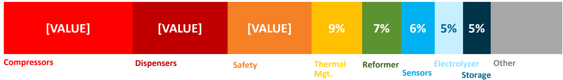
Example: Sources of H 2 Infrastructure Maintenance (out of 5,531 events)
