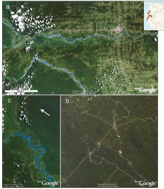
Figure 2.11. (a) In Ecuador, pipelines and roads were built concurrently during the 1960s, leading to colonization and deforestation. (b) In contrast, the remote producing fields in northern Peru were treated like offshore oil platforms; workers were transported by air, and equipment by river barge. (c) As a result, pipeline right-of-ways in Peru (arrow) were not converted into highways, and large scale deforestation has been avoided (Google Earth ™ Mapping Services).
