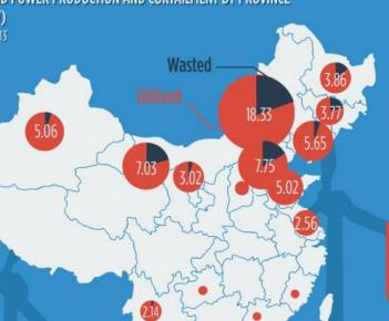
China is the fastest growing market for wind power in the world. But continued growth is hindered by low grid connectivity (wind turbines not physically connected to the power grid) and high rates of curtailment (power grid companies opt to limit the use of wind power due to difficulties in integrating this intermittent power onto the grid). Both issues stem from a lack of planning, insufficient market incentives for power grid companies, and outdated or weak grid technology.
