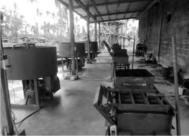
Figure 4. Machines for producing hollow concrete blocks that will be sold to agencies involved in the reconstruction of other cities. Javier, Leyte. Photo: by the author, March 12, 2014.
