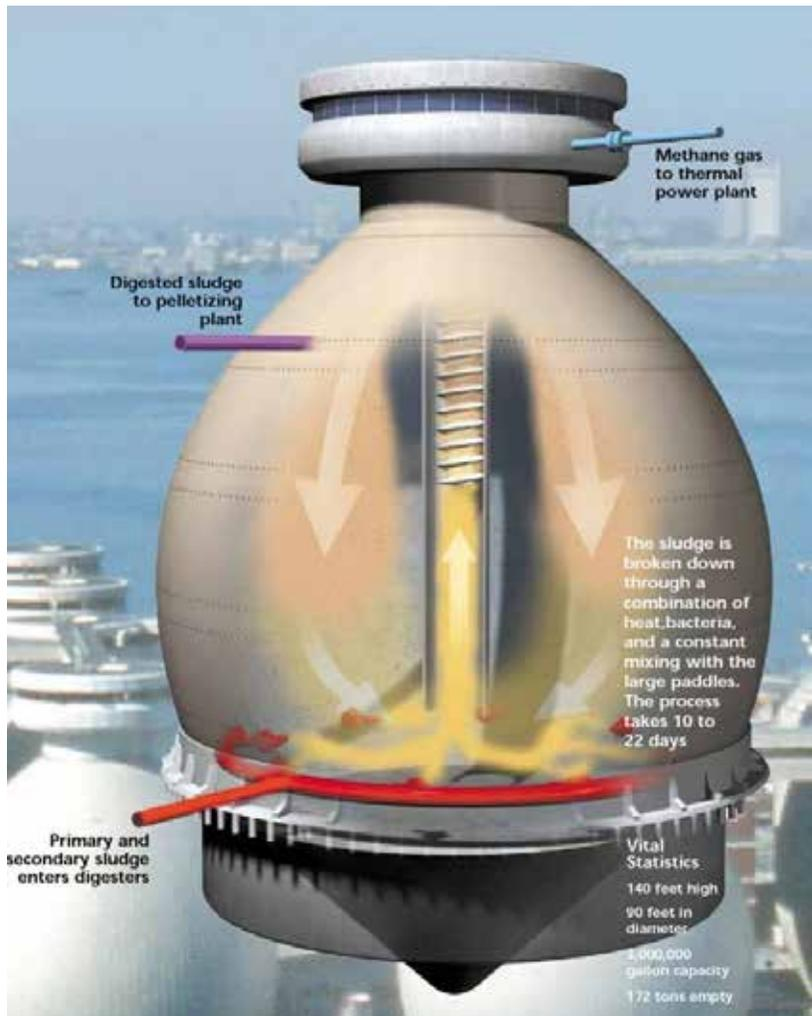
**Figure 2. Anaerobic Digestion:** MWRA uses 12 of these egg shaped digesters in the process
