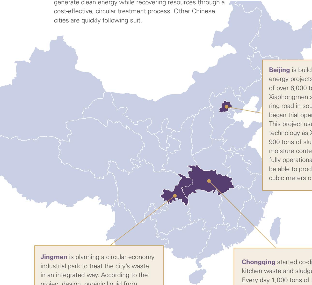
**Beijing** is building five sludge-to-energy projects with a total capacity of over 6,000 tons per day. The Xiaohongmen site, near the fourth ring road in southeast Beijing, began trial operations in July 2016. This project uses the same THP+AD technology as Xiangyang to treat 900 tons of sludge (at 80 percent moisture content) per day. When fully operational, the project will be able to produce 40,000–60,000 cubic meters of biogas.
