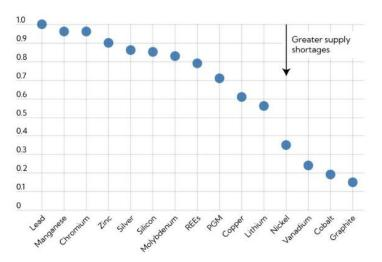
Plot of metals needed for net zero energy transition. A ratio of 0.1 indicates current supply is one tenth the supply needed for this scenario. Source – International Monetary Fund.
